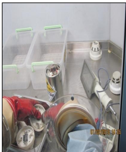
Fig.4. Glove boxes in APLC
