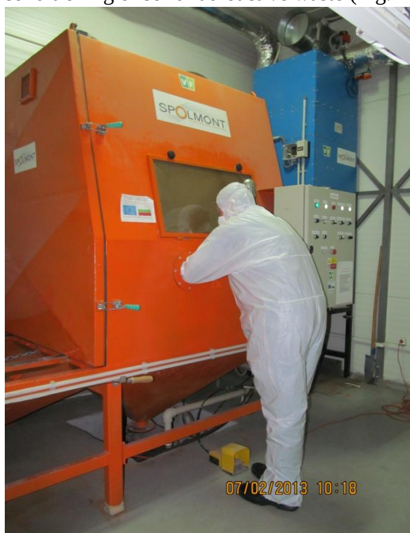
Fig.10 Working chamber of the system for abrasive decontamination
