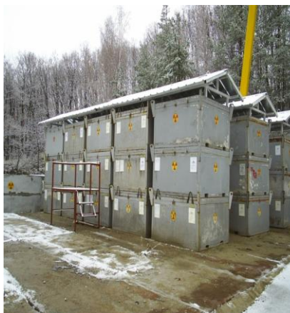
Fig.23 A set of containers type CUBE for temporary storage of radioactive waste, equipped with movable roof
