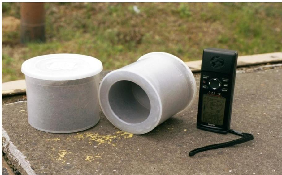
*Figure 7. The most important tools on the field were Marinelli beakers for samples and GPS to mark the locations.*
