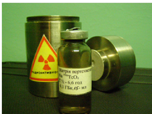
Figure 3. Delivery set of the ^{99m}\text{Tc} -pertechnetate: the flask with the solution of \text{Na}^{99m}\text{TcO}_4 and the transport container (encasement and cover).
