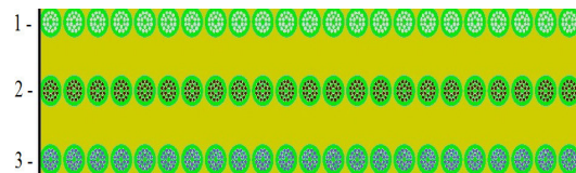
Fig. 3 Part of the design model of SFS-1. Initial enrichment of ^{235}\text{U} in SNF, %: 1-1.8; 2-2.0; 3-2.4
