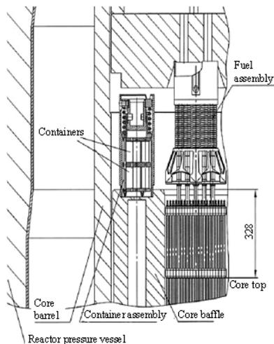
Figure 1. Location of container assemblies in VVER-1000 reactor.
