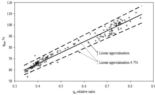
Figure 2. The maximal flux onto PV vs the forward fuel assembly relative power averaged through a fuel cycle for various Ukrainian unit loadings.
